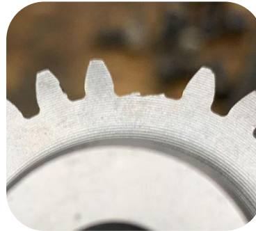
Side profile of gear root failure.
