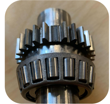
Angled view of gear root failure.
