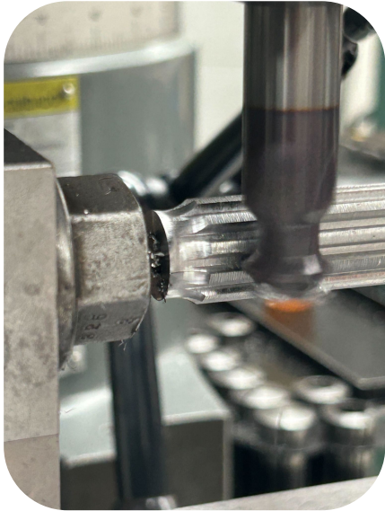
Spline Selection Allows for in House Manufacturing of the Male Input Shaft Spline
