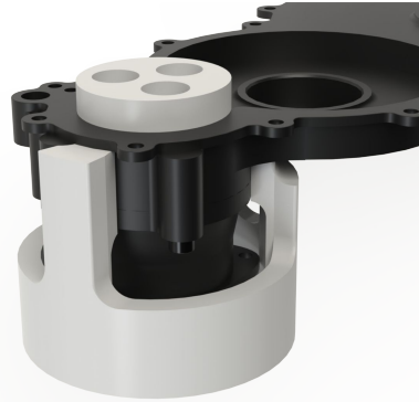
3D Printed Jig to remove third case
