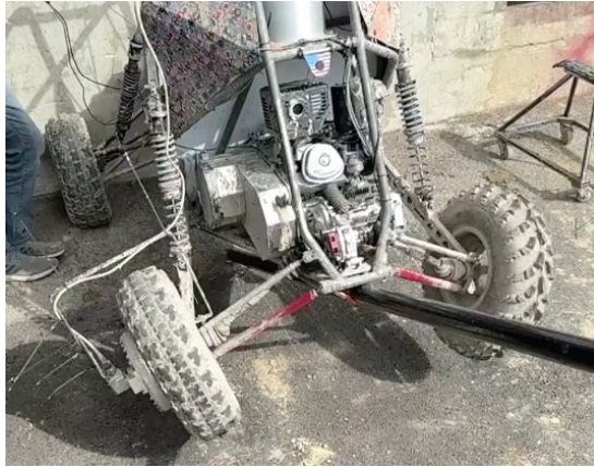
Driveline Drop Test on R24
